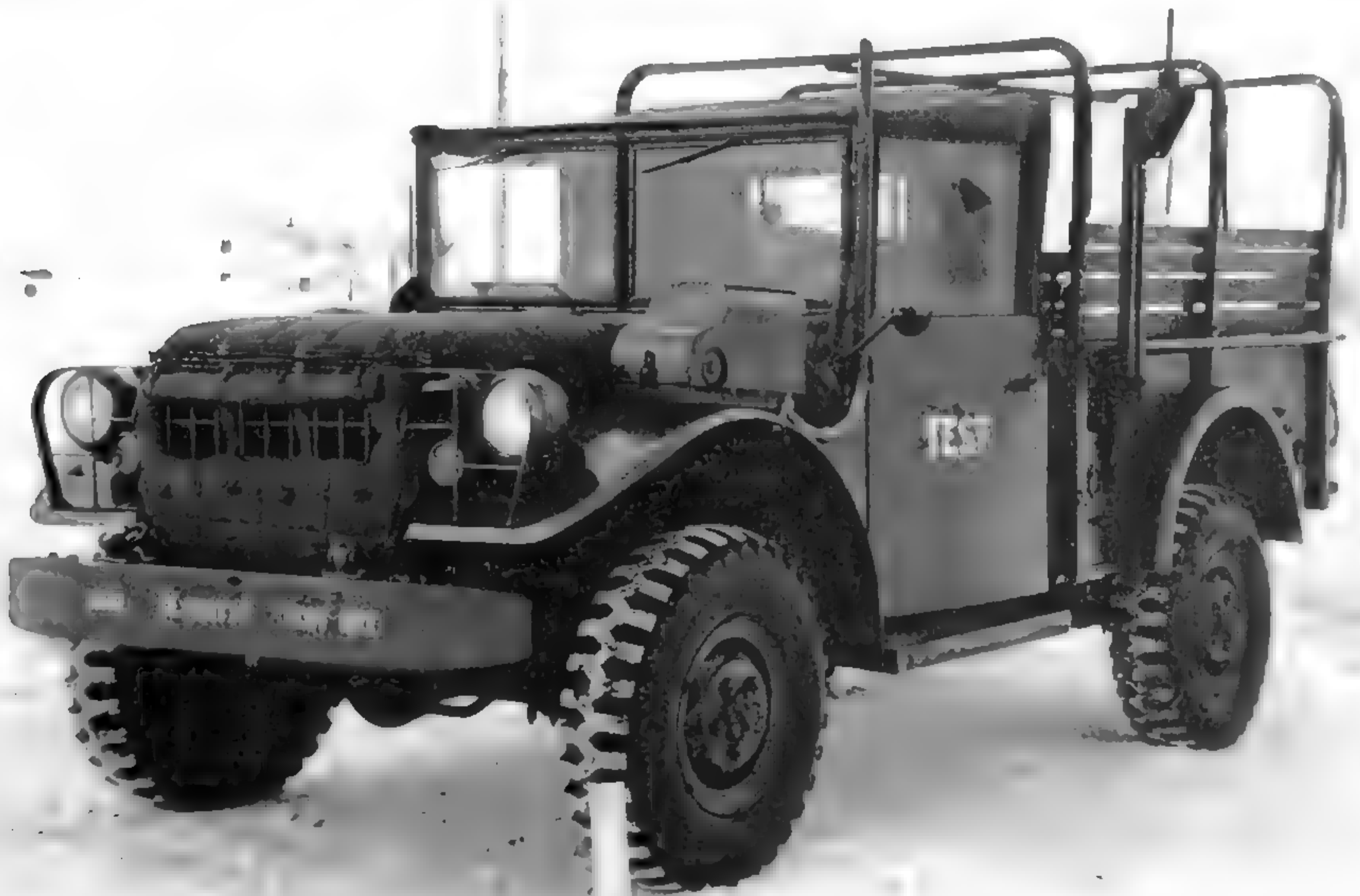
For extreme cold-weather operation, a fuel-fired heater kit was developed for the M37 as well, as is seen in this December 1952 photograph taken during testing at Fort Churchill, Canada. The insulated blanket on the hood, as well as the winter front over the radiator, were a part of this kit, whose heart was the box mounted on the left front fender. For less frigid areas, a hot water-type heater was developed. Although it was shaped differently and lacked the exhaust pipe of the fuel fired heater, it mounted similarly. (National Archives and Records Administration photo)
